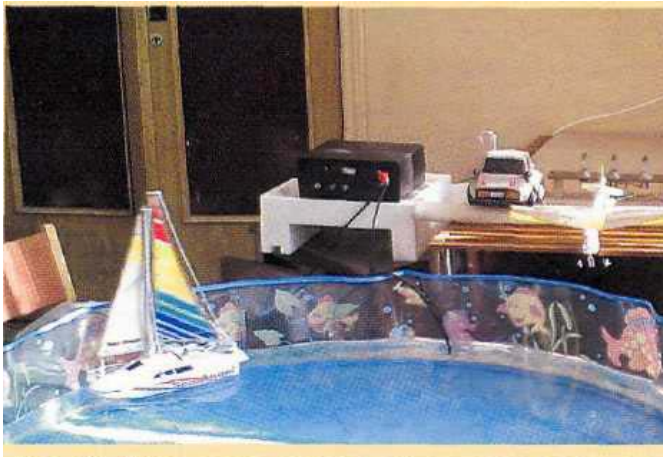
Fig. 9. Electric boat model receiving electric power through the water
