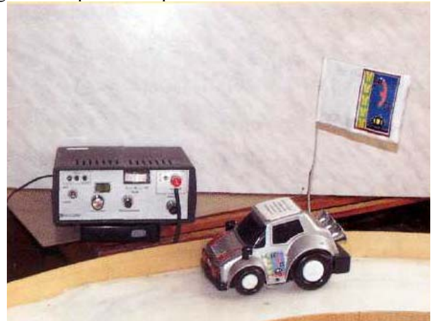
Fig. 10. Contactless high frequency electric vehicle
